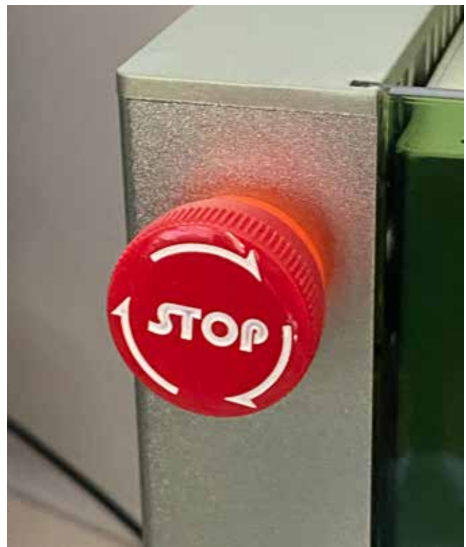
FIG. 12. In case of an emergency, or to abort any operation, the F1 can be stopped immediately by pressing the red Stop button. The button is reset by twisting it to the right.
