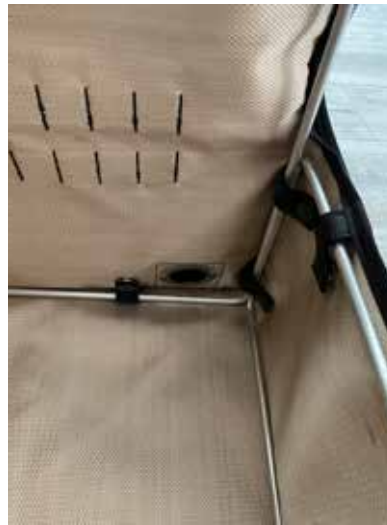
FIG. 9. The Ortur Enclosure 2.0 is assembled by snapping a number of straps around pieces of aluminum framing.
