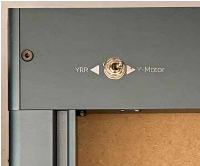
FIG. 6. The new rotary motor vs. Y-axis motor switch simplifies changing from one to the other.
