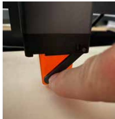
FIG. 7. The easily accessible focus lever provides an exact measurement between the laser beam and the work object.
