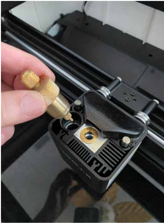
FIG. 13. In this photo, with the M1 turned upside down, the blade cutter is being removed prior to the installation of the air assist nozzle. When the blade cutting function is to be used, this opening is where the cutter is installed. Ordinarily the blade cutter is installed with the M1 in its upright position.
