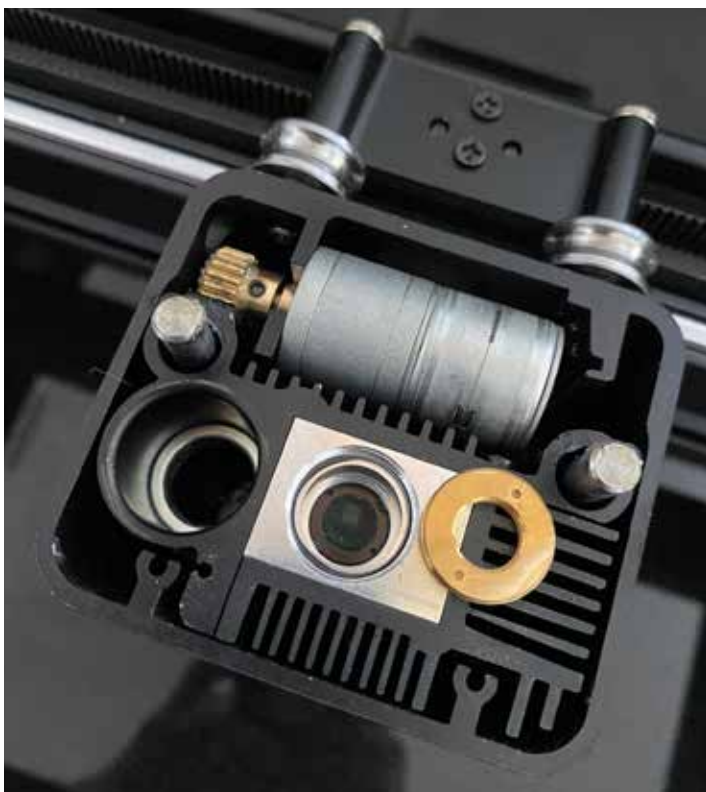
FIG. 4. The original laser lens mount, shown immediately to the right of the laser lens, is removed using a double-pronged tweezers provided with the air assist kit.
