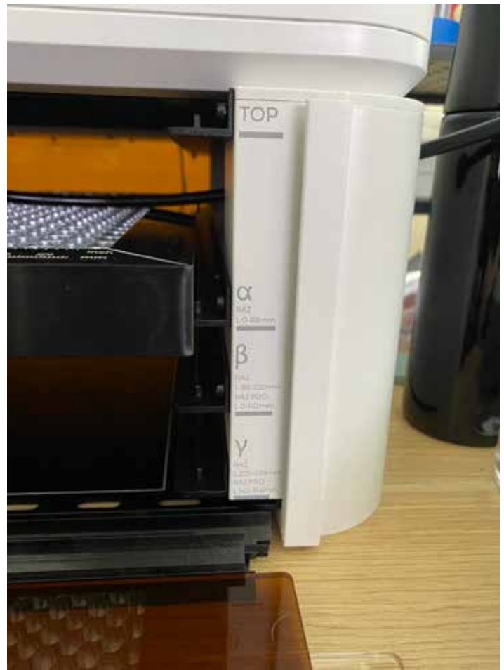
FIG. 8. The Riser Base is segmented into three heights, labeled with the Greek characters alpha, beta, and gamma (A, B, and C). These characters are related to the distance of the honeycomb panel surface to the laser.
