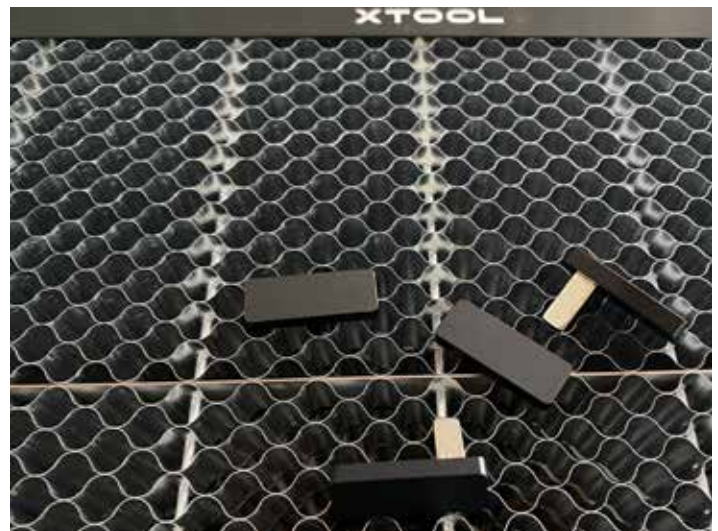
FIG. 9. The magnetic material pins shown sitting on top of the honeycomb panel. The silver protrusions fit snugly into the honeycomb cells.
