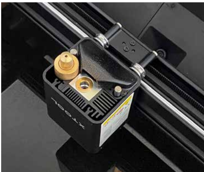
FIG. 3. The laser module prior to any modifications. Note that both the laser and the knife cutter are in place. As set, the knife cutter would be active.
