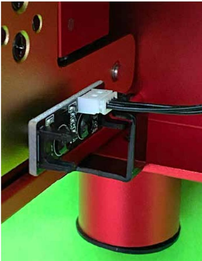
FIG. 11. xTool uses an advanced design, long-lasting electronic limit switch, which is superior to a mechanical roller lever arm.
