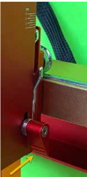
FIG. 7. The release lever on the right side of the laser module is used to set the position of the laser height (z-axis) for cutting, using the increments inscribed in white on the upper edge.
