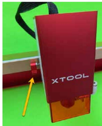
FIG. 2. The locking mechanism on the left side of the laser module secures the position of the unit on the z-axis. The lever is an improvement over the original design first shipped with the D1.
