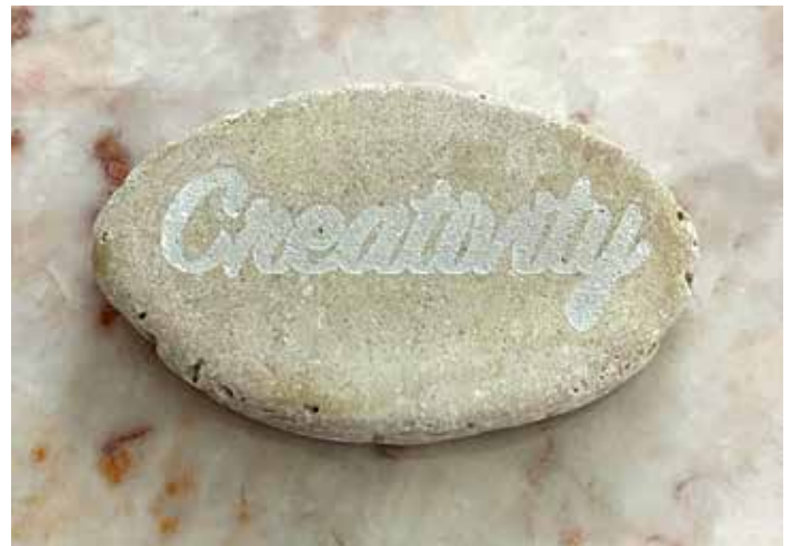
FIG. 8. This stone was engraved without the use of any pre-treatment. After processing the user has the option of adding color to improve the contrast of the lettering.
