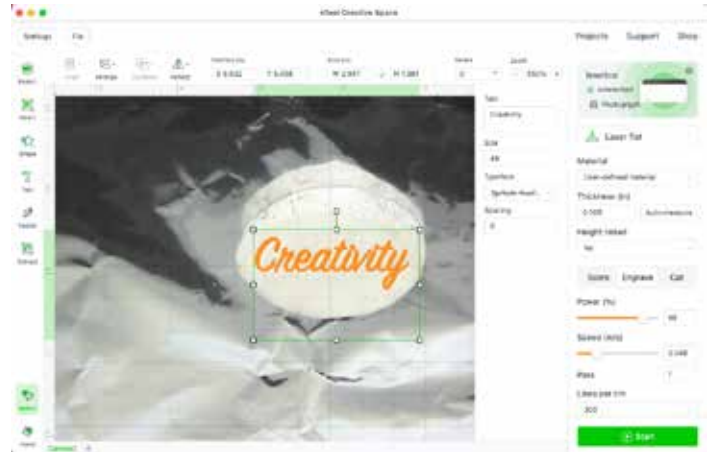
FIG. 7. In the work area the user has placed a piece of aluminum foil, shiny side up, to prevent stray laser movement from hitting the laser bed and leaving an unwanted image. The text tool has been used to type the word "Creativity," with the user's choice of typeface. The user positions the word in the required position and selects the Engrave option.
