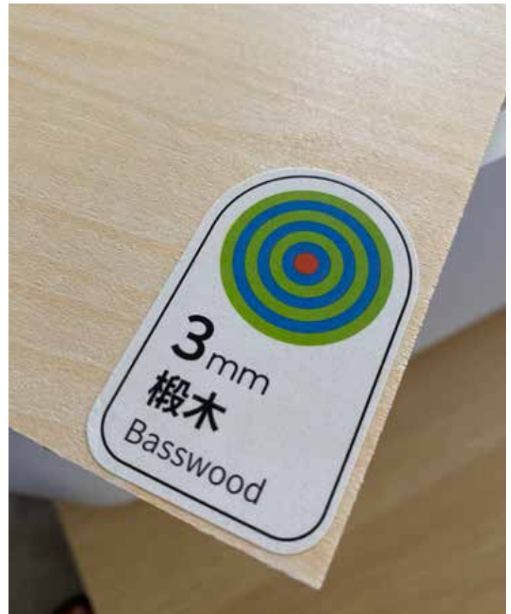
FIG. 5. A ring code is provided on all xTool-supplied materials to provide the M1 with relevant information regarding material characteristics and processing requirements.
