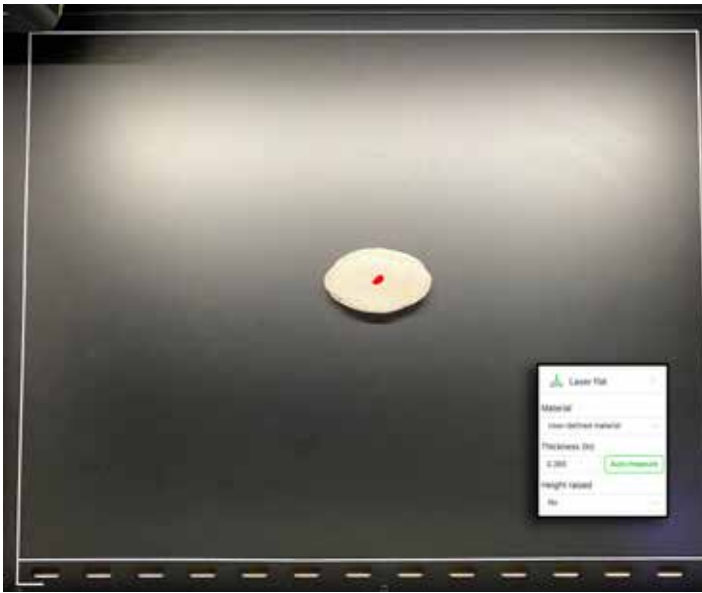
FIG. 6. Here a flat rock has been placed on the workbed. The red spot that appears in the center of the rock is the laser that is determining its thickness by using the Auto-measure button in the Creative Space software (inset).
