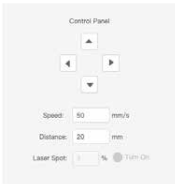
FIG. 9. The user can define the incremental movement of the laser head as it frames its intended image
